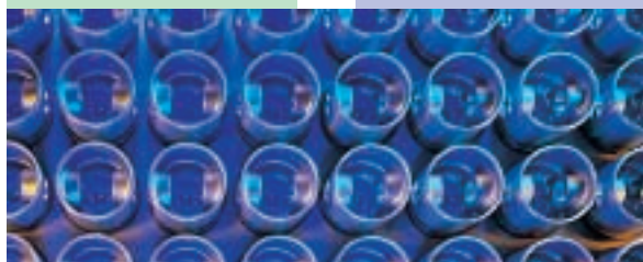
The pistons, one of the most important parts of the reciprocating compressors. They pump the refrigerant, e.g. ammonia, through the installation. In this way "cold" can be produced.
