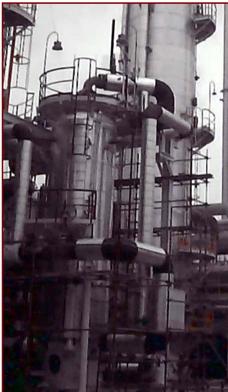
FIG. 7 - New Axial-Radial Pre-reformer in Ultrafertil Cubatao
