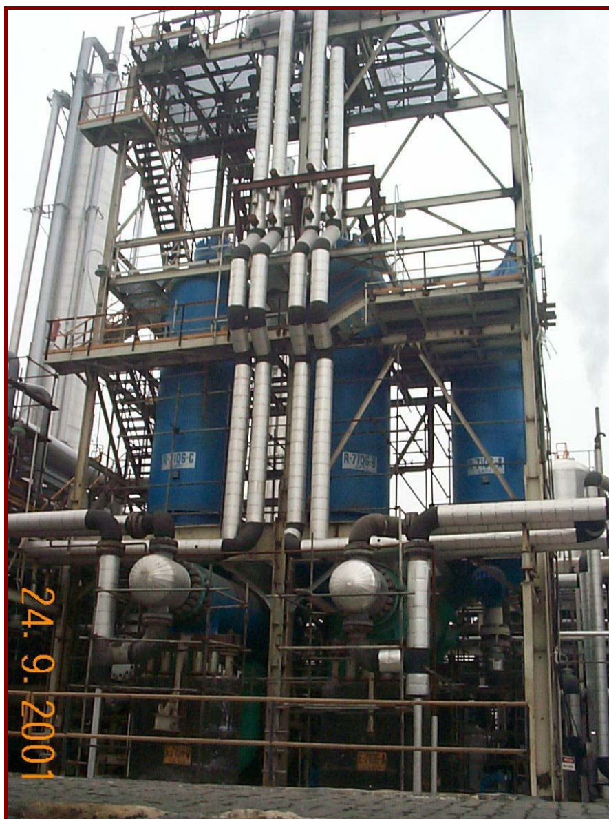
FIG. 8 - New Ammonia Synthesis Converters at Ultrafertil Cubatao
