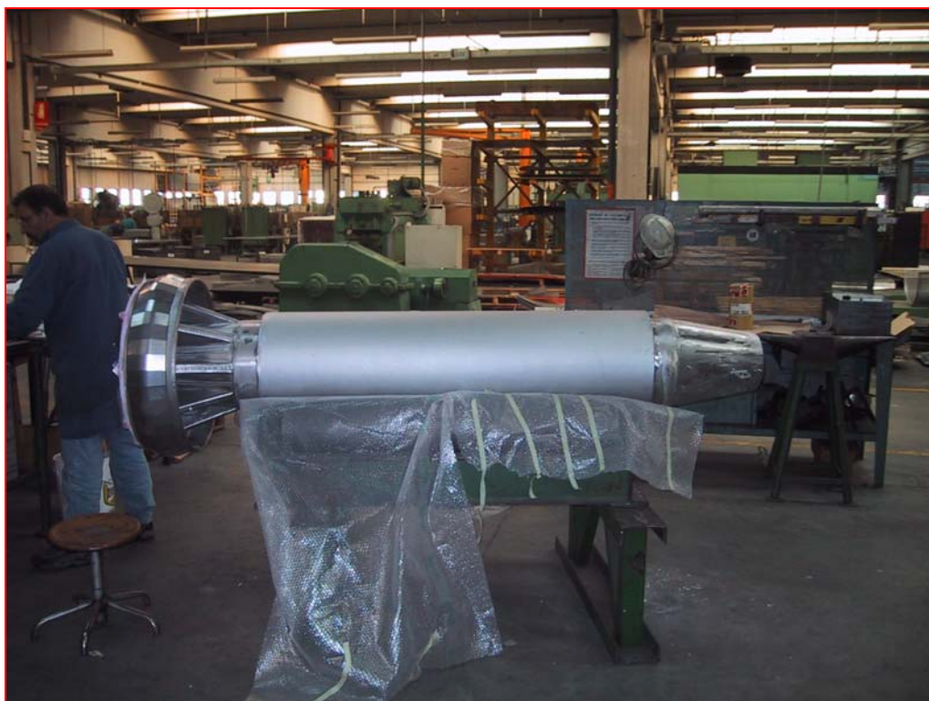
Fig. 4 – CASALE Secondary Reformer Burner
