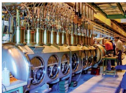
The cryogenic systems of the superconducting dipole magnets were tested here before being installed in the LHC tunnel"
